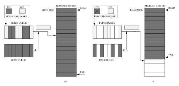
Figure 6: Foreground thread flushing mechanism - (a) a reorder buffer full of foreground thread instructions and with a cache-missing load at its head triggers a flush, and (b) state of the buffers after flushing. Dark shaded blocks denote foreground thread instructions, while light shaded blocks denote background thread instructions.
