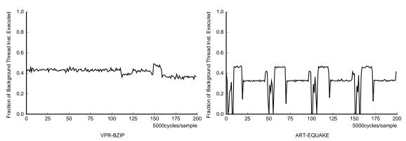
Figure 13: Histogram of the fraction of executed instructions from the background thread when running simultaneously with a single background thread. This fraction of executed instructions from the background thread is averaged over an interval of 5000 cycles.
