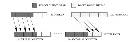
Figure 5: Slot Prioritization with the ICOUNT.2.N fetch partitioning mechanism. (a) First, the foreground thread is allocated all the fetch slots it needs. (b) Then, the background thread is allocated the remaining fetch slots.
