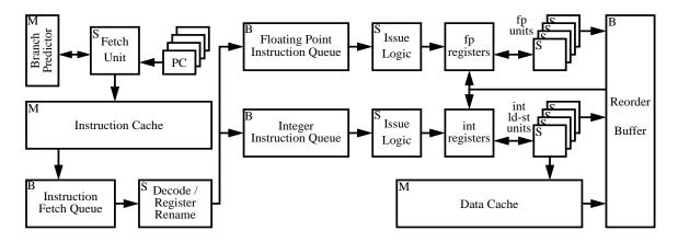
Figure 2: SMT processor hardware (diagram adapted from [1]). Each shared hardware resource is labeled with a letter signifying one of three resource classes: instruction slots (S), instruction buffers (B), and memories (M).
