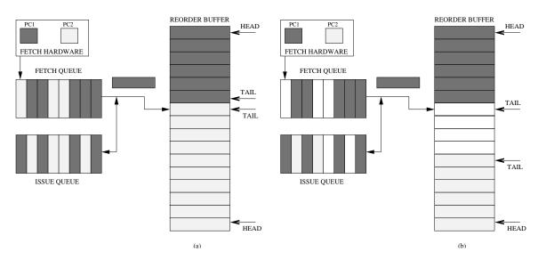
Figure 4: Background thread flushing mechanism - (a) collision between background and foreground threads in the reorder buffer triggers flushing, and (b) state of the buffers after flushing. Dark shaded blocks denote foreground thread instructions, while light shaded blocks denote background thread instructions.
