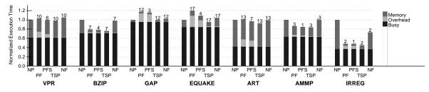
Figure 19: Normalized execution time for different prefetching schemes: no prefetching (NP), naive conventional software prefetching (PF), selective conventional software prefetching (PFS), Transparent Software Prefetching (TSP), and TSP without foreground thread flushing (NF). The label appearing above each bar reports the number of instrumented loops.
