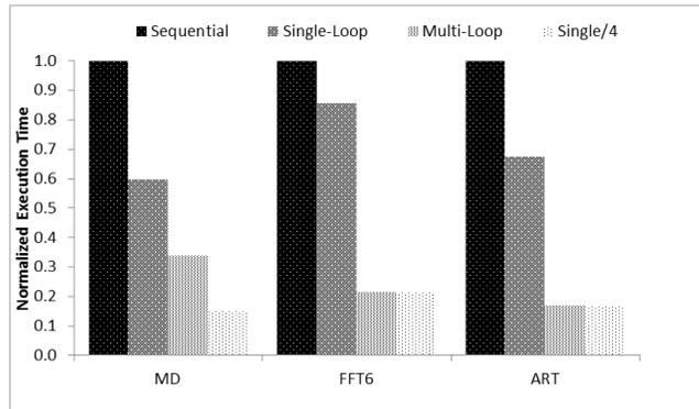
Fig. 3. Normalized execution time for sequential, single-loop and multi-loop parallelism, and multi-loop parallelism without contention.
