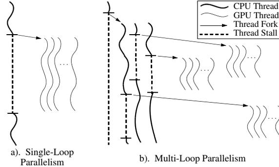
Fig. 1. CPU and GPU threads in a). single-loop and b). multi-loop parallelism.
