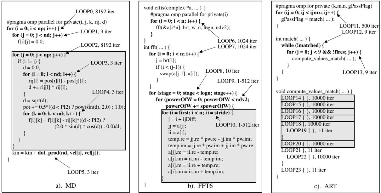
Fig. 2. Code examples from the a). MD, b). FFT6, and c). ART benchmarks exhibiting multi-loop parallelism. Our technique schedules the parallel outer loops (OpenMP pragmas) on CPUs, and the parallel inner loops (shaded gray) on GPUs.
