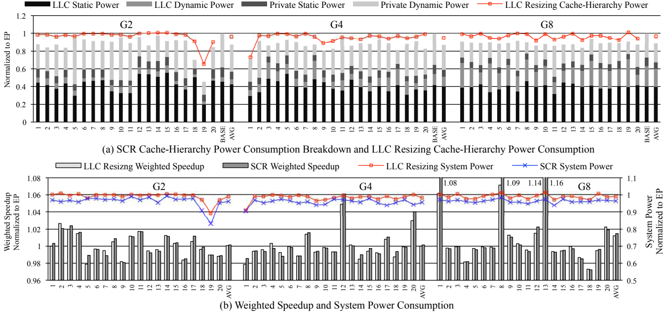
Figure 6: Power consumption and performance of dynamic SCR and LLC resizing.
